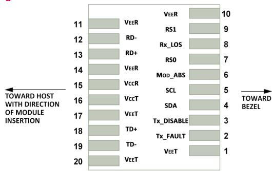
Host PCB SFP+ Pad Assignment Top View
